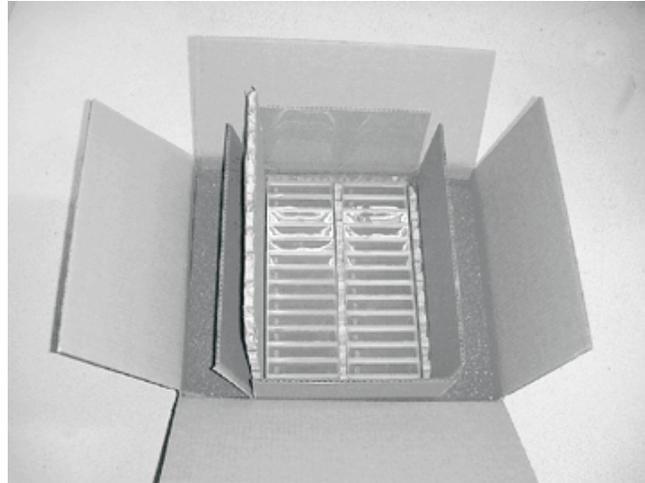
Figure 48. Double-boxing tape cartridges for shipping
