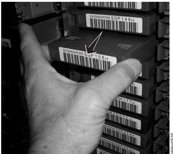
Figure 38. LTO cartridge removal from an HD slot
