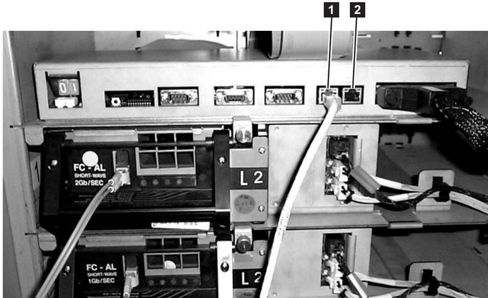
Figure 84. Medium changer assembly. The MCA is located above the drives and the power trays, and is part of the enhanced frame control assembly power structure.
