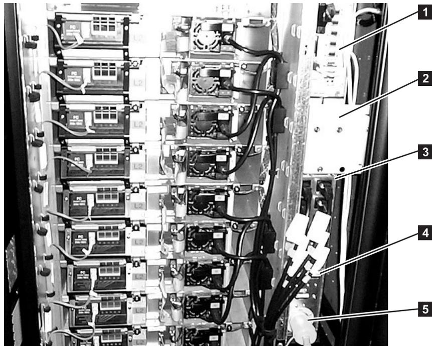
Figure 73. Components of the frame control assembly. Located at the right rear of the , this power structure comes with models L25, D25, L55, and D55. A model L52 frame is shown.
