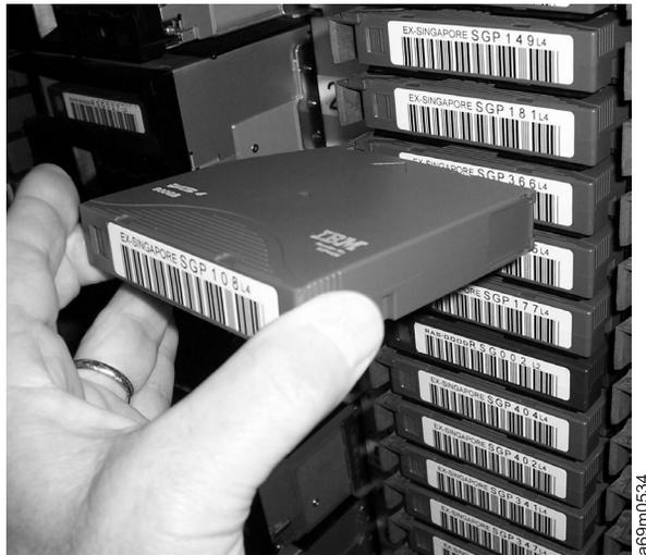
Figure 39. LTO cartridge removed from an HD slot
