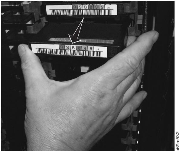
Figure 41. 3592 cartridge removal from an HD slot
