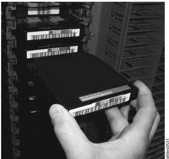
Figure 42. 3592 cartridge removed from an HD slot
