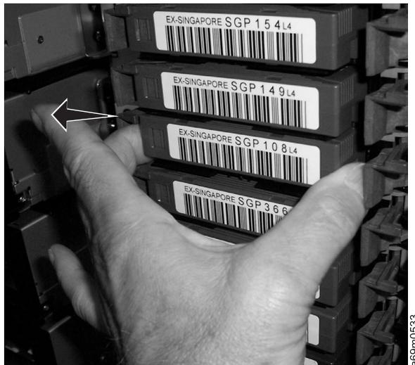
Figure 37. LTO HD slot gate release
